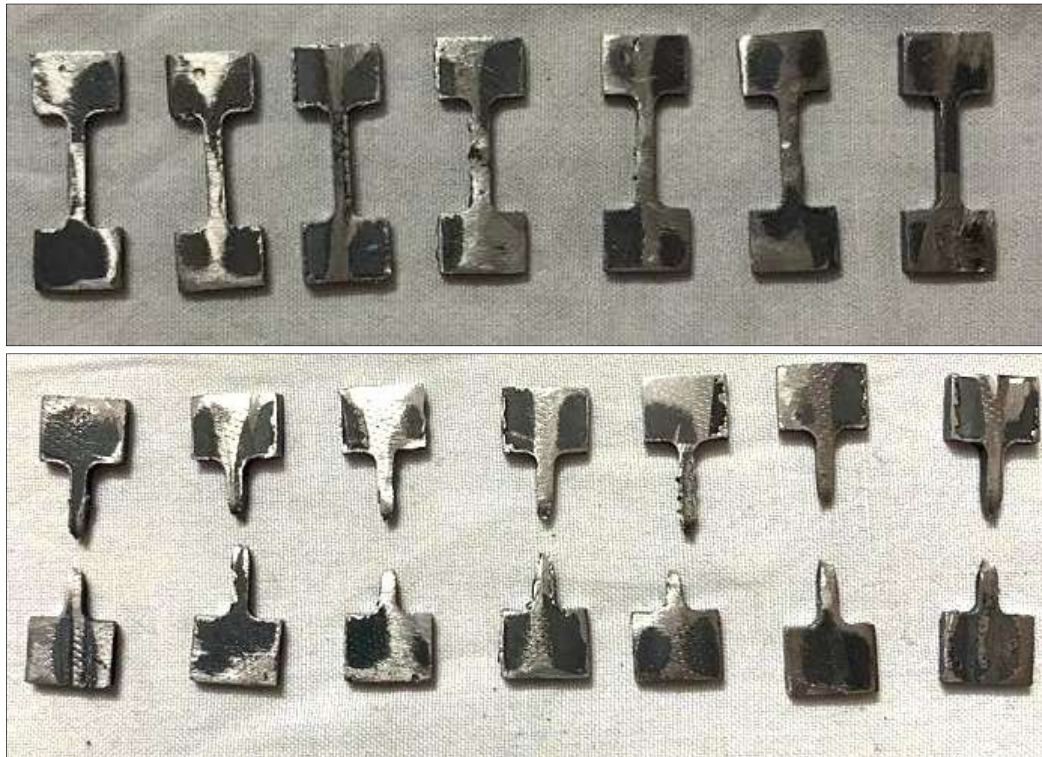
Fig. 4.23. Before and after testing tensile test specimens.
