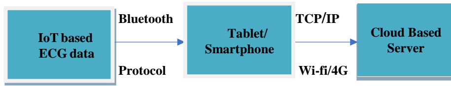
Figure 4.21 IoT-based system diagram with sensors, electrocardiogram machine, and smartphone [Reproduced from S. Kumari et.al, 2018]
