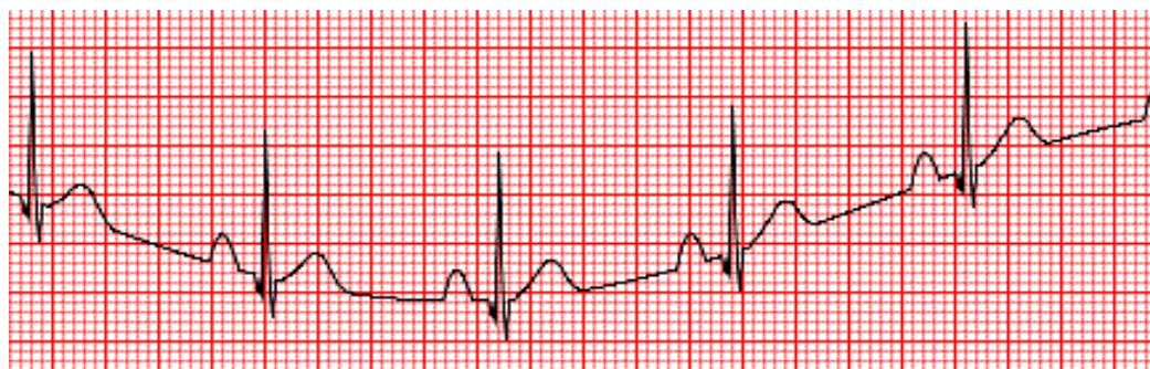
Figure 1.6: Baseline wander Noise [reproduced from http://www.mauvila.com/ECG/ecg_artifact.htm ]
