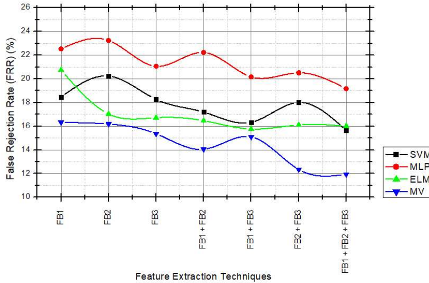
Figure 5.9: Illustration of false rejection rate (%) vs. feature extraction and classification techniques considered
