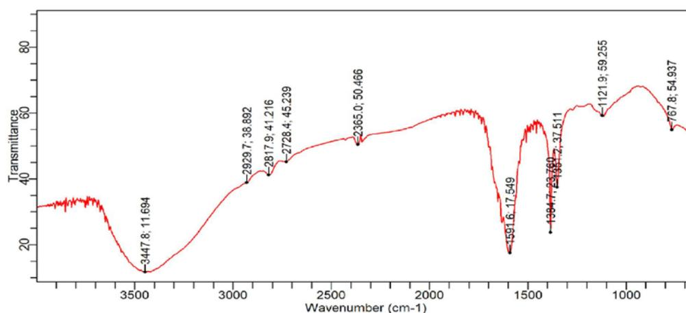
Figure 4.1: FTIR spectrum of Mesalamine.
