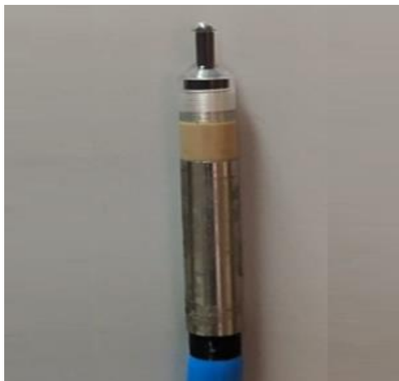
Figure 2.4: PinPoint ionization chamber
