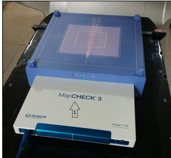
Figure 2.10: MapCHECK 3 diode array
