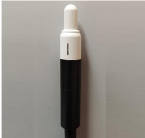
Figure 2.3: SNC125c ionization chamber
