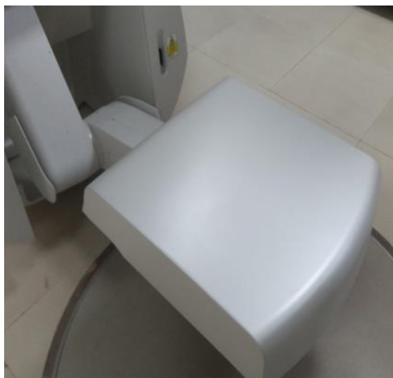
Figure 2.11: Electronic portal imaging device based portal dosimetry system
