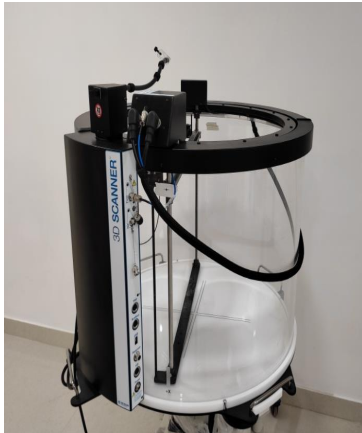
Figure 2.2: Sun nuclear three dimensional (3D) scanner water phantom
