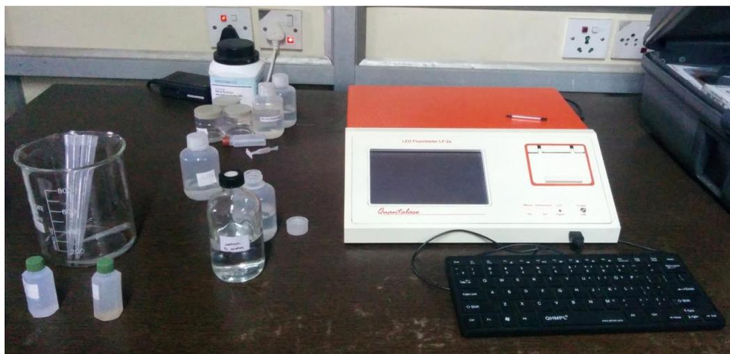
**Figure 2.12:** LED Fluorimeter along with accessories
