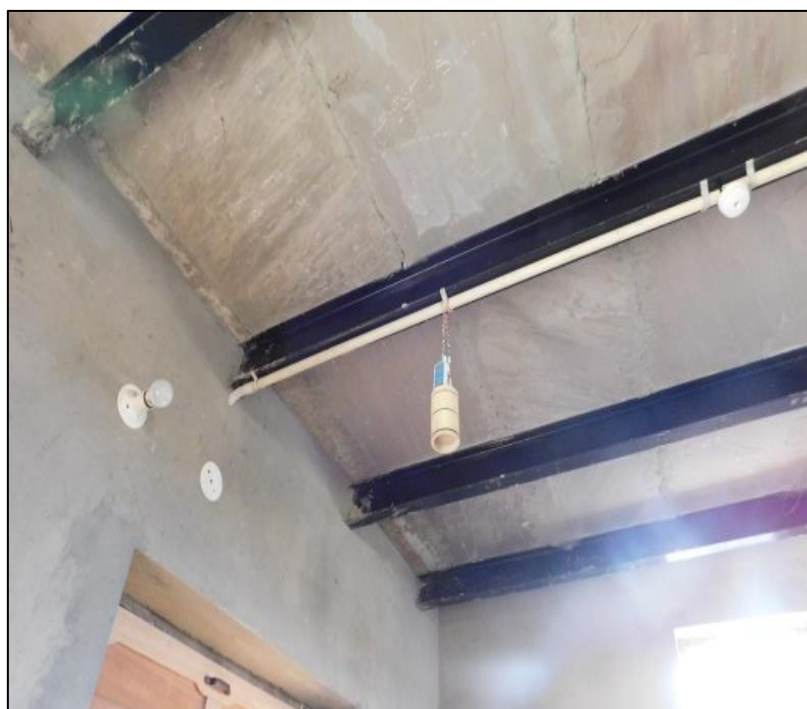
Figure 3.1: Deployed dosimeters, DRPS/DTPS and wiremesh in the dwellings
