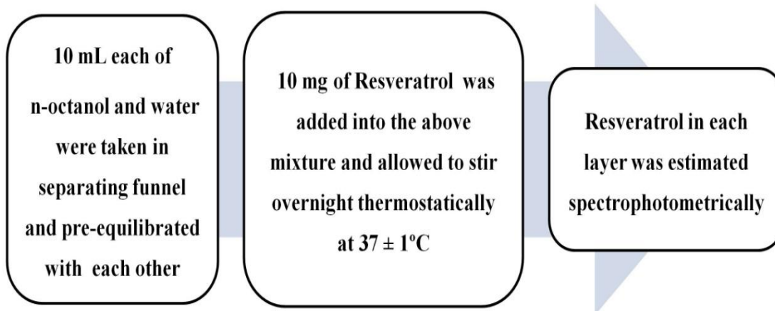
Figure 4.7: Schematic representation of the procedure for determining the partition coefficient of Resveratrol
